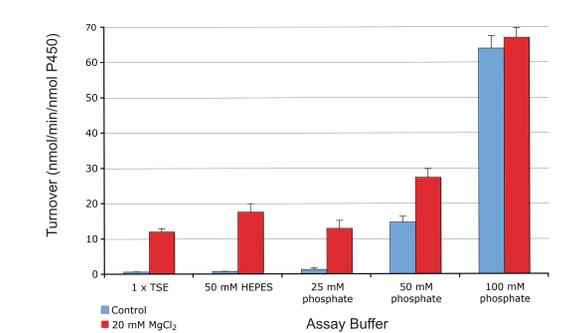
Fig 3a. Effect of MgCl<sub>2</sub> on testosterone turnover by CYP3A4R Bactosomes.
